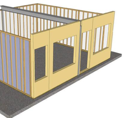
The options to fix cladding, both internally and externally, to anywhere on the SIP means that almost any option can be considered, with hanging weights of up to an impressive 50kg/M2 easily achievable.
